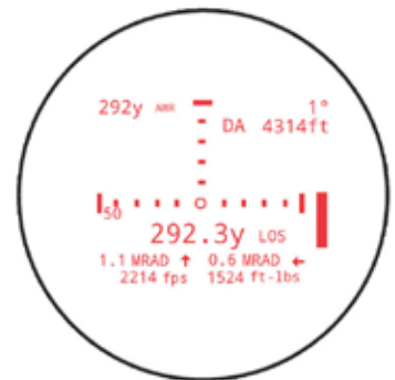
Active-Matrix OLED display for graphical real-time ballistic information
